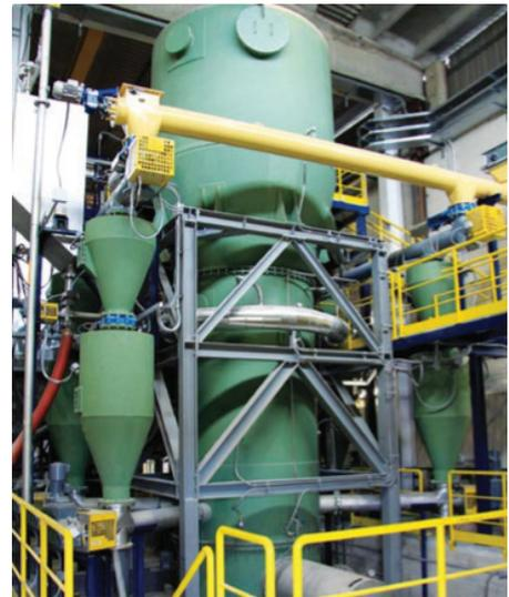
**Fluidised bed gasifier using EQTEC gasifier technology**
